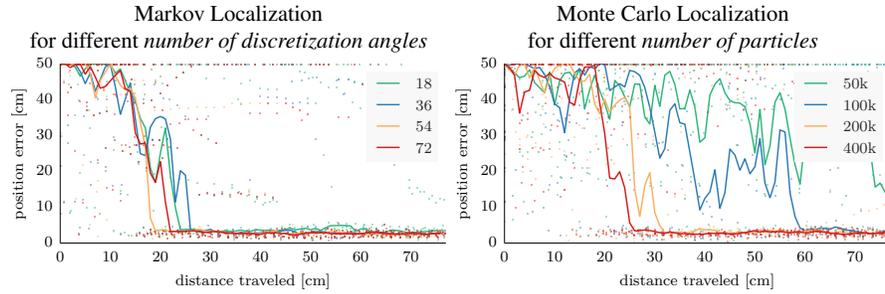
**Fig. 3** The error between the estimation by the localization algorithm and the ground truth on 10 segments from the first two trajectories. The solid lines show the median while the light dots show the individual trials.
