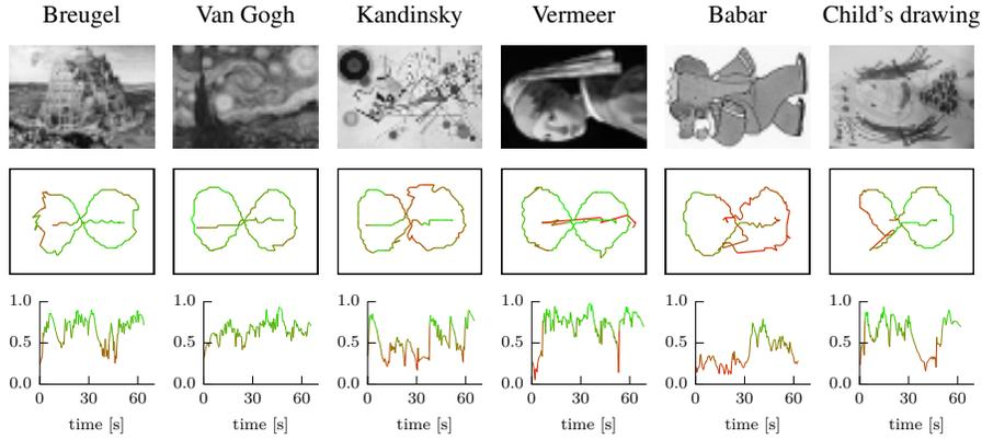
**Fig. 6** The image, estimated trajectory and self confidence for different  $59 \times 42$  cm grayscale patterns printed on A2 papers with a resolution of 1 pixel/cm. The robot is remotely controlled to draw a 8-shape figure, with similar motor commands for each image. Markov Localization with 36 discretization angles used. The color of the lines vary from red (confidence 0) to green (confidence 1). Trajectories are plotted starting from a confidence level of 0.2.
