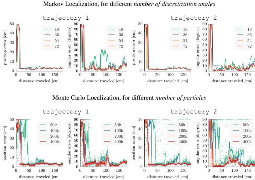
**Fig. 2** The error between the estimation by the localization algorithm and the ground truth on trajectory 1 and trajectory 2. For Monte Carlo Localization, the solid lines show the average over 10 trials, while the light dots show the individual trials.
