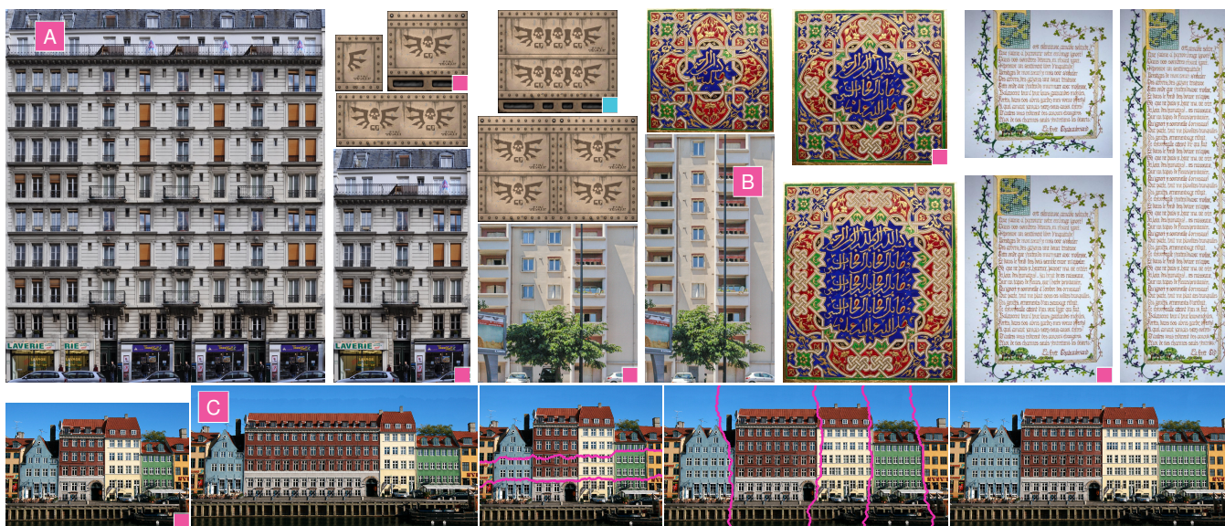
Figure 7: Top: Synthesis results. Source images are marked with a pink square. The histogram window size parameter \xi is 250 for the leftmost image. Drag-and-drop control is used on the image marked with a blue square. Bottom, left to right: The Copenhagen harbor. Automatic enlargement. 2 control cuts (in pink) to add one floor. 4 control cuts to set the building sizes. Final result.
